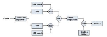
A group of registers starts with a **Condition register**. An internal **Event** will set the corresponding bit of the Condition register (to 'set a bit' means a transition from binary **0** to a binary **1**). Any Condition register will be updated continuously. This means that a bit will be reset as soon as the condition which rose that bit is no longer valid.
